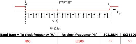
$Rx \ clock = \frac{1}{78.125 \times 10^{-6}} = 12800 \rightarrow Tx \ clock = \frac{12800}{16} = 800$  $12800 = \frac{24 \times 10^{6}}{SBR} \rightarrow SBR = 1875 = 0x0753$
